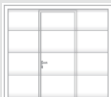
Symmetrical arrangement for garage door widths up to 3.50 m
